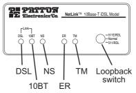
Figure 12. Model 1082 front panel
